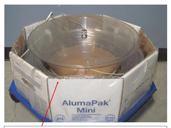
Pak-Extender removed to show the inside of the mini-drum when set-up properly with the Pak-Feedassist-A located in the short fiber ring at the bottom.
